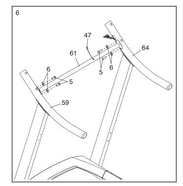
7. With the help of a second person, hold the console assembly near the Right Handrail (64).
